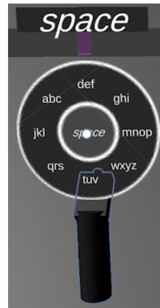
Figure 3: The default design of VRKeyboard. Note that the white circle indicates the joystick's current orientation and the black textbox above the keyboard that corresponds with the key the joystick is currently highlighting
