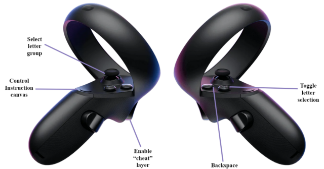
Figure 6: A visualization of the control scheme of VRKeyboards, both non-cheat and cheat.
